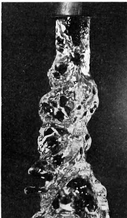
How water flowing freely from a faucet looks, when photographed in the light of the Edgerton stroboscope, which can take 6,000 pictures per second by means of electron tubes
